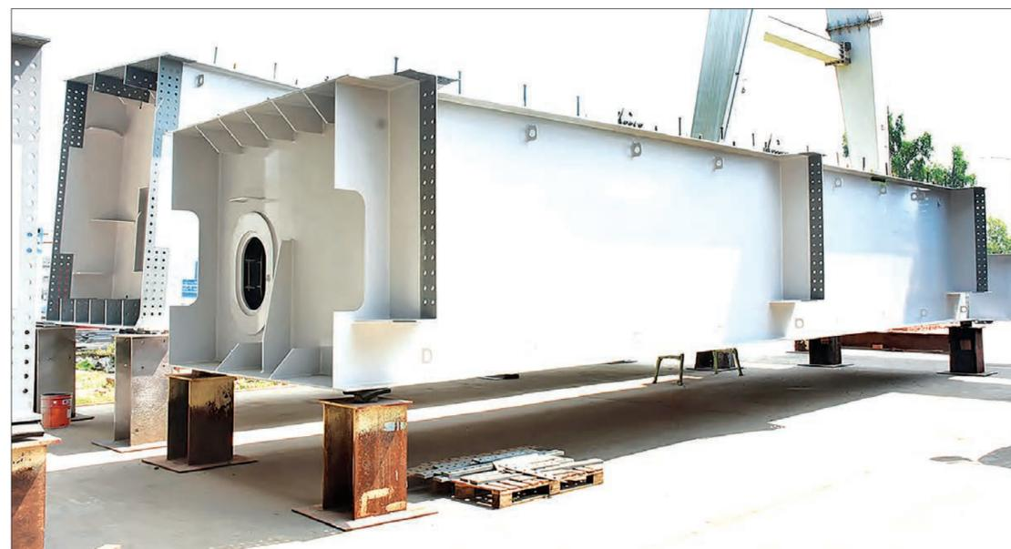
Steel frames produced by J&M Factory.
